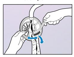
A nylon brush is the most effective when cleaning the Filter Basket. Using a nylon brush, hold the Filter Basket under running water and brush from the inside of the basket out. Always treat the Filter Basket with care; it can be easily damaged.  Discoloration of the plastic may occur with some fruit and vegetables. To help prevent this, wash all parts immediately after use.
